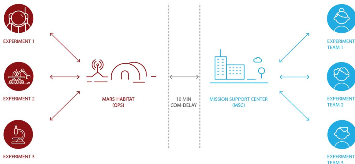
**Figure 1.** Conceptual architecture of the AMADEE-20 expedition: A 10min time delay reflects the signal travel time between Earth and Mars. The Mission Support Center in Innsbruck/Austria is the single-line-of-contact between “Earth” and “Mars”.
