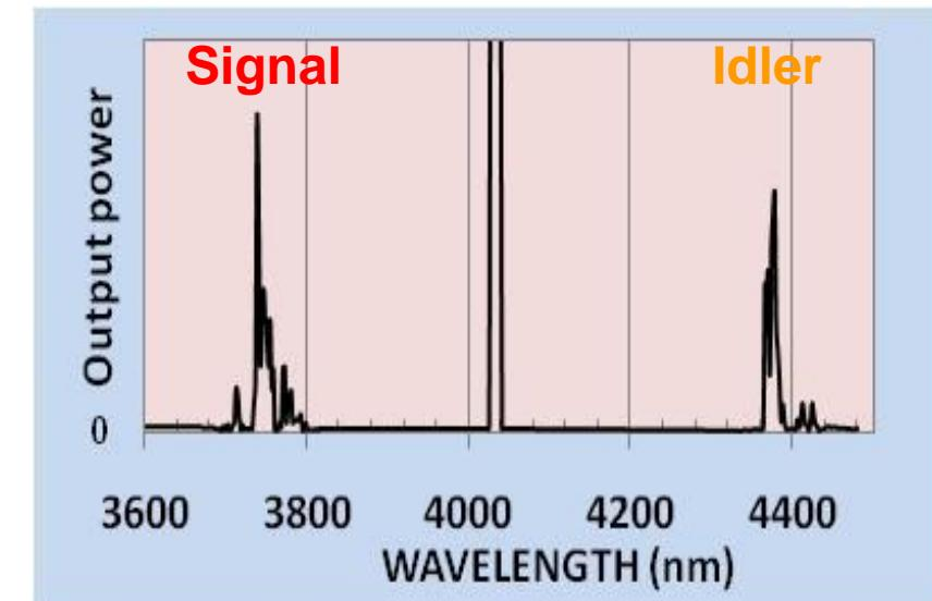
Parametric power spectral scan
