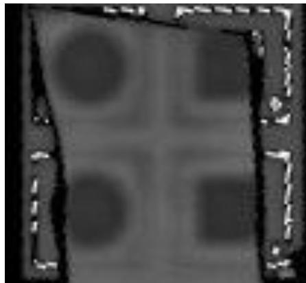
Acoustic Microscope image is used to analyze the wafer bonding
