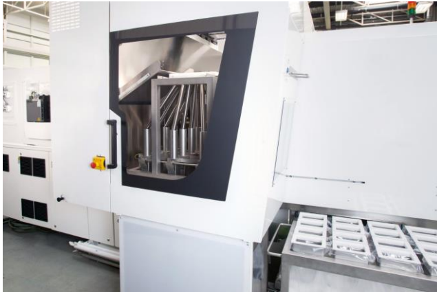
Compact integration: The pipe distributor fits in the machine's safety guard.
